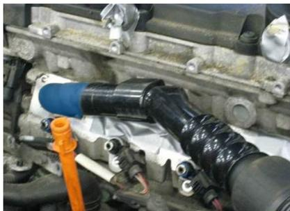
7. Adjust the cylinder to be cleaned to Top Dead Centre to ensure the valve is closed. **Note. Cleaning may only be carried out with the valves shut.**
